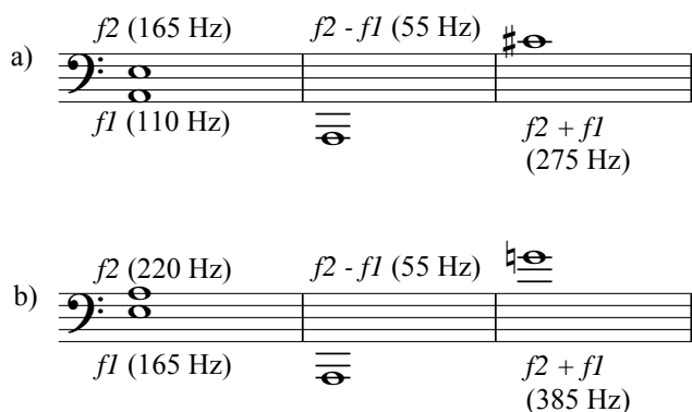
Example 2.3. The simplest difference and summation tones of the fifth A-e (a) and the fourth e-a (b).
