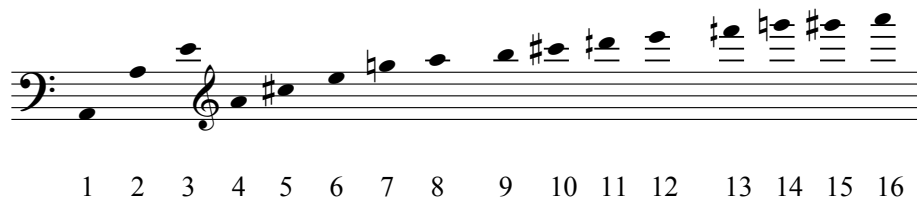
Example 2.2. The first 16 partials of the harmonic series of A (110 Hz) (an approximate, equal-tempered notation). The frequency of a harmonic is 110 Hz multiplied by the harmonic's number.
